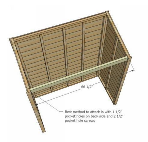
The easiest solution for the walls is to purchase several fence panels. Simply create posts at the corners of your shed and along the sides if it is larger than one panel.
