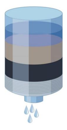
In a biofilter, water moves through three layers to filter your water.
